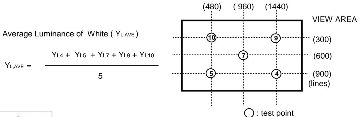
Note 5) After stabilizing and leaving the panel alone at a given temperature for 30 min , the measurement should be executed. Measurement should be executed in a stable, windless, and dark room. 30 min after lighting the backlight. This should be measured in the center of screen.
