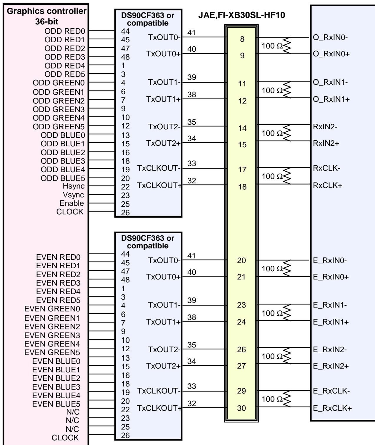
Note : The LCD Module uses a 100ohm resistor between positive and negative lines of each receiver input.
