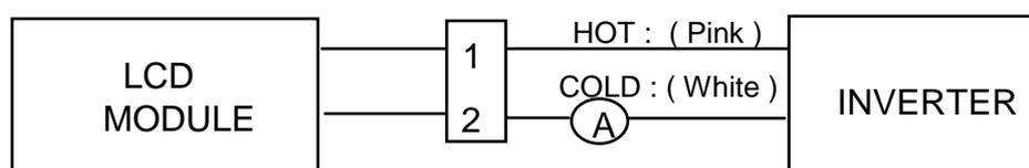
(2) Lamp frequency may produce interference with horizontal synchronous frequency and this may cause line flow on the display. Therefore lamp frequency should be detached from the horizontal synchronous frequency and its harmonics as far as possible in order to avoid interference.
